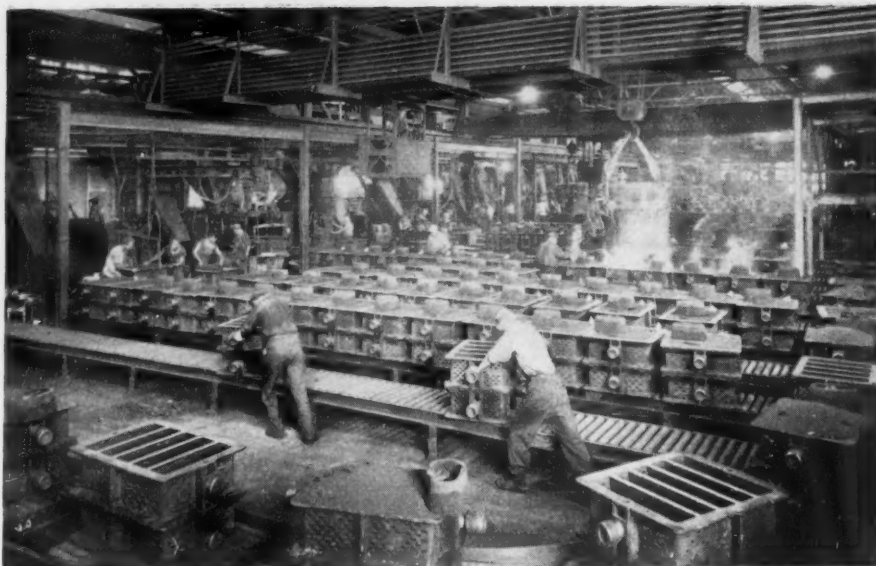
Highly-mechanized section of the molding floor at the Crane Co., Chicago, foundry is shown above. Molding machines are shown at left rear. Molds are poured on the stationary roller conveyors, then pushed off onto the power-driven mold conveyor shown in foreground. The two workmen are returning empty flasks to the molding machines
